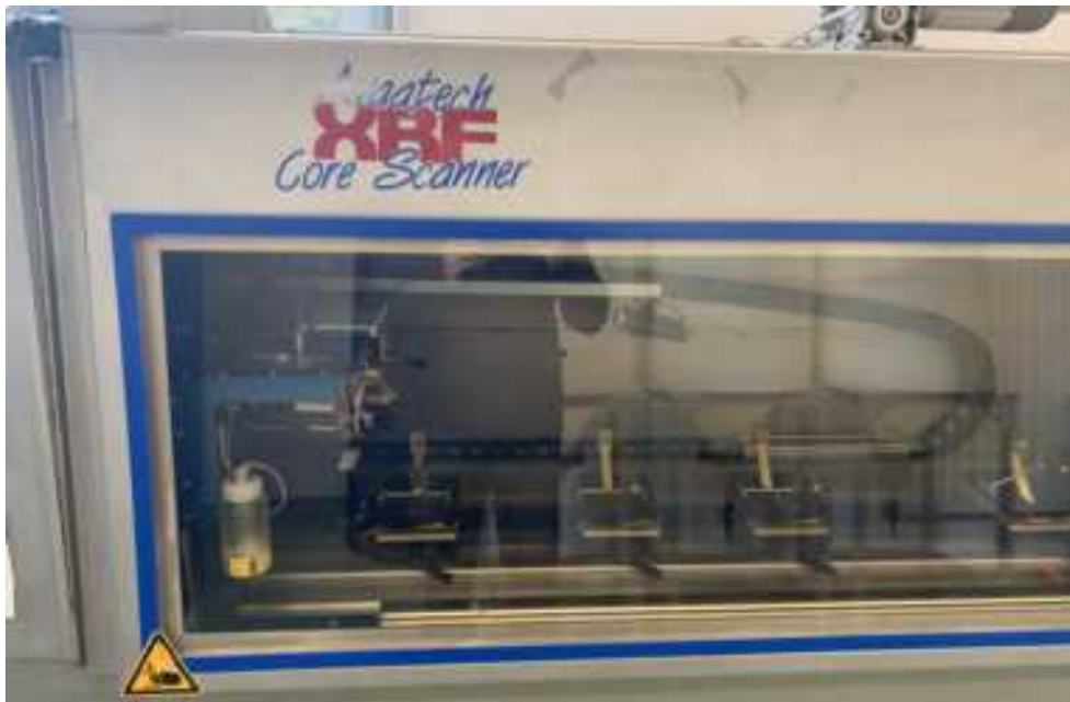
Figure 3.2: Avaatech micro XRF core scanner in the lab of Eawag for XRF analysis.
