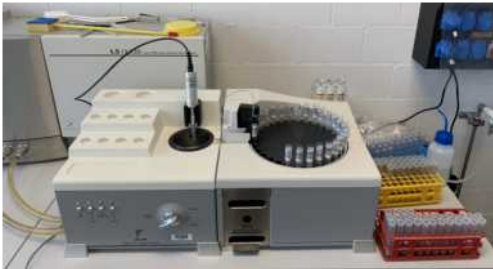
Figure 3.3: Photo of LS 13 320 XR Laser Diffraction Particle Size Analyzer (Beckman & Coulter) used for the analysis.
